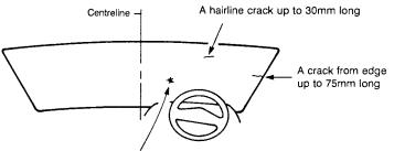
A 'bullseye' crack up to 16mm diameter
