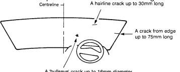
A 'bullseye' crack up to 16mm diameter
