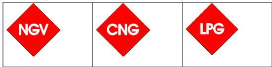
White lettering on red background. Labels are to be a minimum of 25mm x 25 mm in size. Letters must be capitals and of a minimum of 6mm in height.
