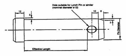
Material - Steel 4140 (Alternative 4150) (Metric Grade 10.9) - Ultimate Tensile Strength 1040 MPA)
