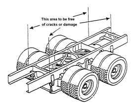
e) Any vehicle wheelbase that has been lengthened or shortened without certification of compliance with section H and C of VSB-6 in the form of a modification plate and Compliance Certificate from a Registering Authority or the NHVR.
