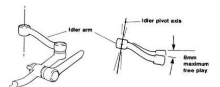
p) Free play at the steered road wheel rim in a horizontal or vertical plane (excluding any necessary wheel bearing play) exceeds manufacturer's specifications. Where these specifications are not known or are no longer appropriate, free play exceeds the amount in the following table:
