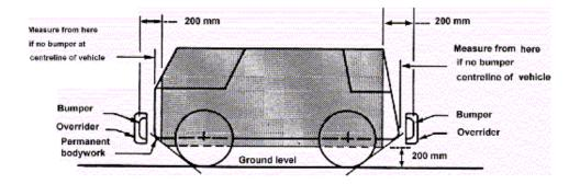
On vehicles with 4.5 tonnes or more tare mass, or where the chassis has more than 600mm ground clearance at the rear:
