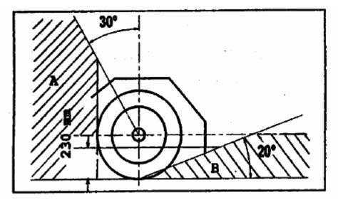
The mudguards on a single axle trailer must provide continuous protection, for the overall width of the tyres, between a point in area A and a point in area B as shown.
