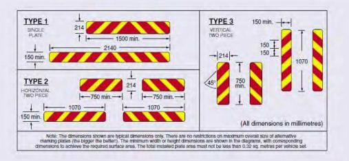
Apart from the dimensions and design, alternative style marking plates must meet all of the requirements for the preferred square plates, including the use of approved retroreflective material and words.
