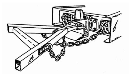
All fixed or rigid pig trailers with a GTM greater than 2.5 tonnes and fitted with automatic pin couplings, all medium and heavy category pig trailers with rigid drawbars and any other trailers without breakaway brakes require safety chains.
