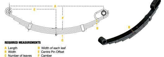
NOTE – WHEN MEASURING THE LENGTH OF A SPRING MEASURE STRAIGHT ACROSS THE SPRING – DO NOT FOLLOW THE CURVE
