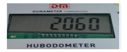
These 4 digital number for the circumference is millimeter (mm). For example, this hubodometer the first circumference is 2060mm, and you want change to your need circumference.
