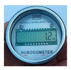
2) Use 2 magnet bars supplied to touch "U" and "E": 'HUBODOMETER' at the same time for 5 seconds to start.
