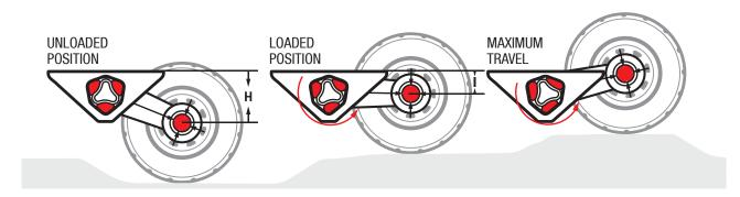
AL-KO's Independent Rubber Suspension axle system is extensively used in a range of applications, from off-road to marine and heavy-duty trailers.
